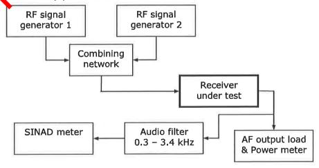
2.2.12.1 Switch the RF signal output of signal generator 2 off.
