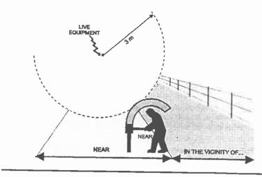
GRAPHIC ILLUSTRATION OF WORKING TO CLEARANCE FROM EXPOSED "LIVE" HIGH-VOLTAGE EQUIPMENT
