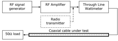
2.4.4.1.1 Tune the RF signal generator to the in-band transmitting frequency.
